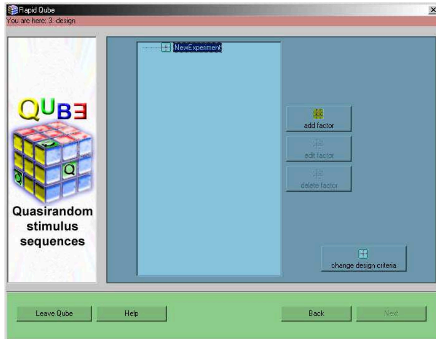
Figure 2.2: The GUI of RQUBE displays three areas of major importance: (1) the navigation bar (red area); (2) the working area (blue); and (3) the button bottom (green).
